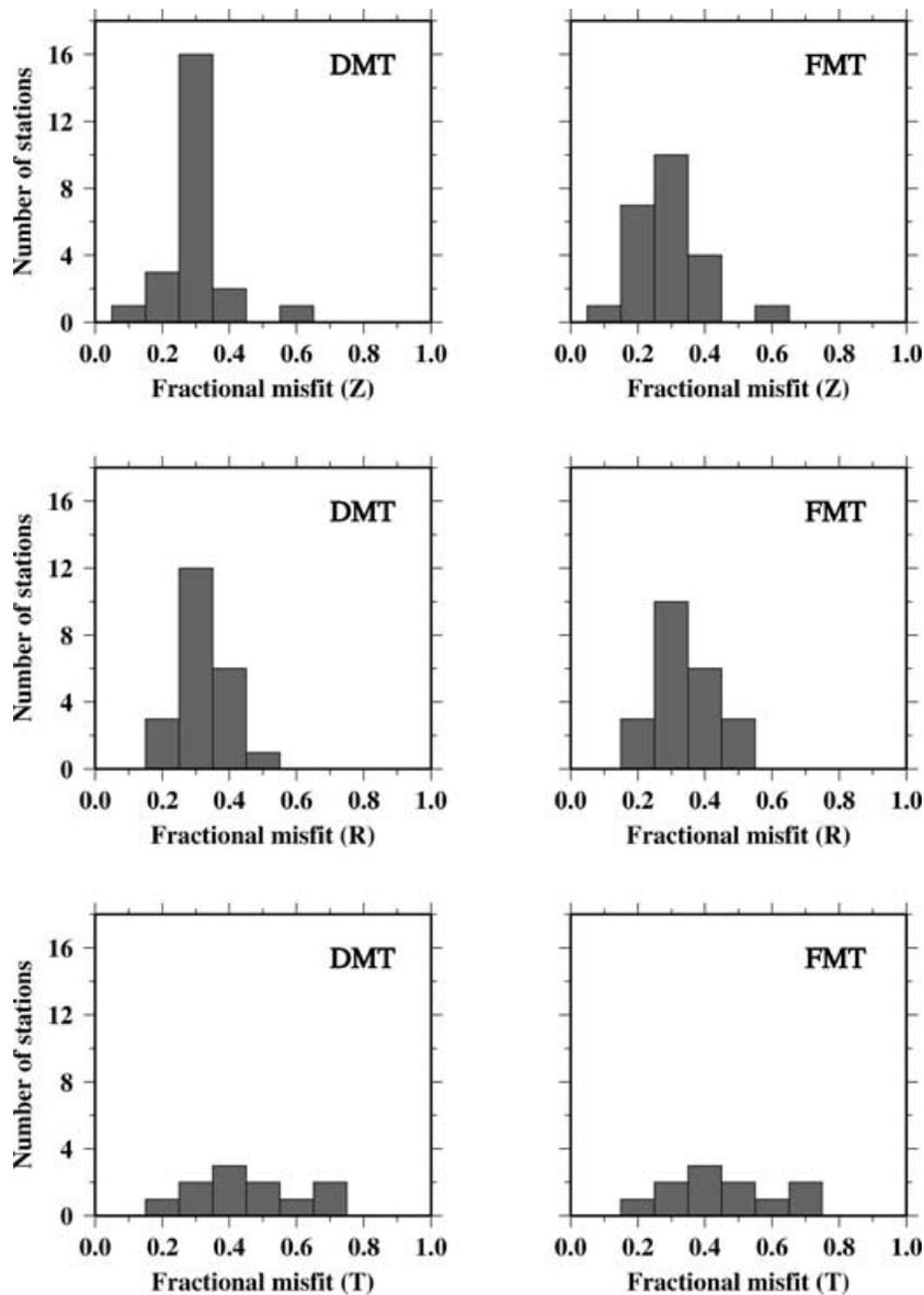
**Figure 7.** Histograms showing the distribution of the fractional misfits for each component (Z, vertical; R, radial; T, transverse) at all HOTSPOT stations for the inversion at 3.5 km depth (DMT, deviatoric moment tensor; FMT, full moment tensor) without distance-dependent weighting. The small number of transverse components is a result of many of them being excluded from the inversion because of contamination with long-period noise.
