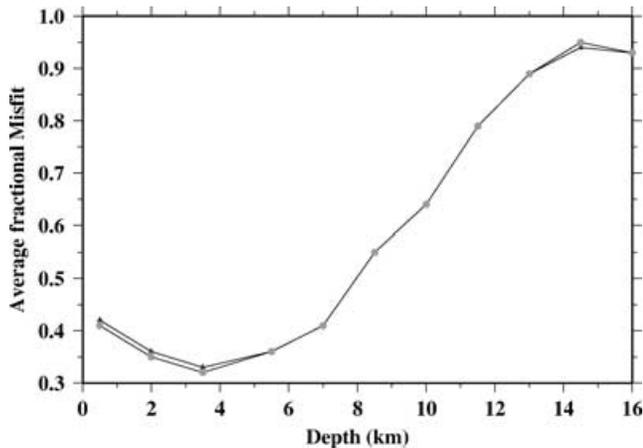
**Figure 6.** Average fractional misfit-versus-depth curves resulting from the inversions of all the available HOTSPOT data. Black triangles indicate the misfits when the inversions were performed without distance-dependent weighting of the data. Grey circles indicate the misfits when the inversions were performed with distance-dependent weighting.
