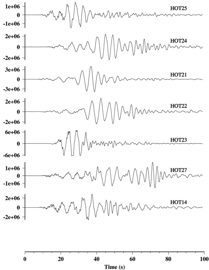
**Figure 3.** Vertical component velocity waveforms of the Bárðarbunga earthquake recorded at the closest (<150 km) HOTSPOT stations. The seismograms are arranged in order of increasing azimuth around the source (amplitudes in arbitrary units). Note the emergent onset and low-frequency content apparent at all stations around the source.
