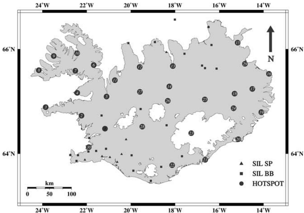
**Figure 2.** Map showing the locations of temporary (HOTSPOT) and permanent (SIL) seismic networks that were operational at the time of the Bárðarbunga earthquake (SP, short-period stations; BB, broad-band stations).
