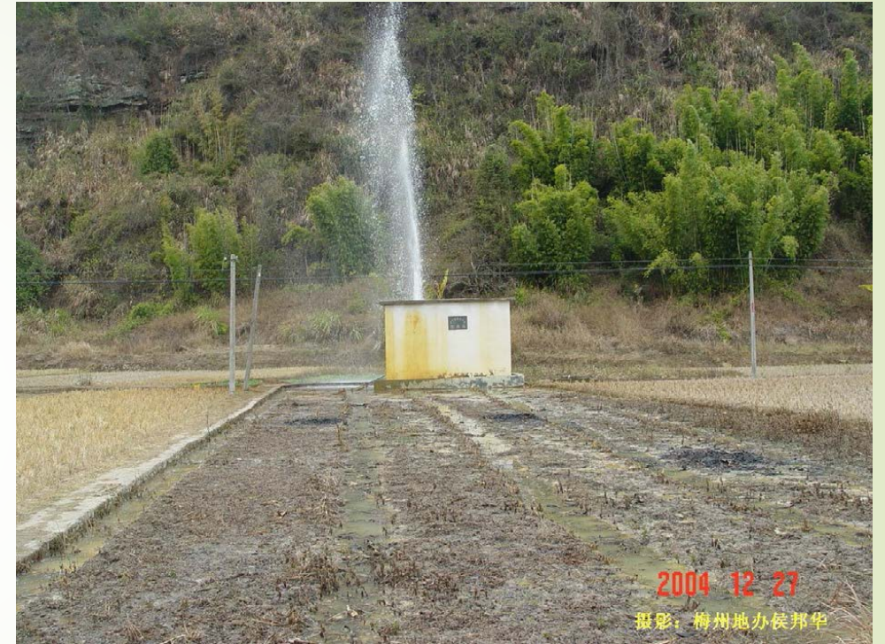
Well in China responding to the December 26, 2004, M 9.2 Sumatra earthquake 3200 km away. The picture was taken by Hou Banghua, Earthquake Office of Meizhou County, Guangdong, 2 days after the Sumatra earthquake. The fountain was 50 – 60 m high when it was first sighted 1 day after the earthquake
