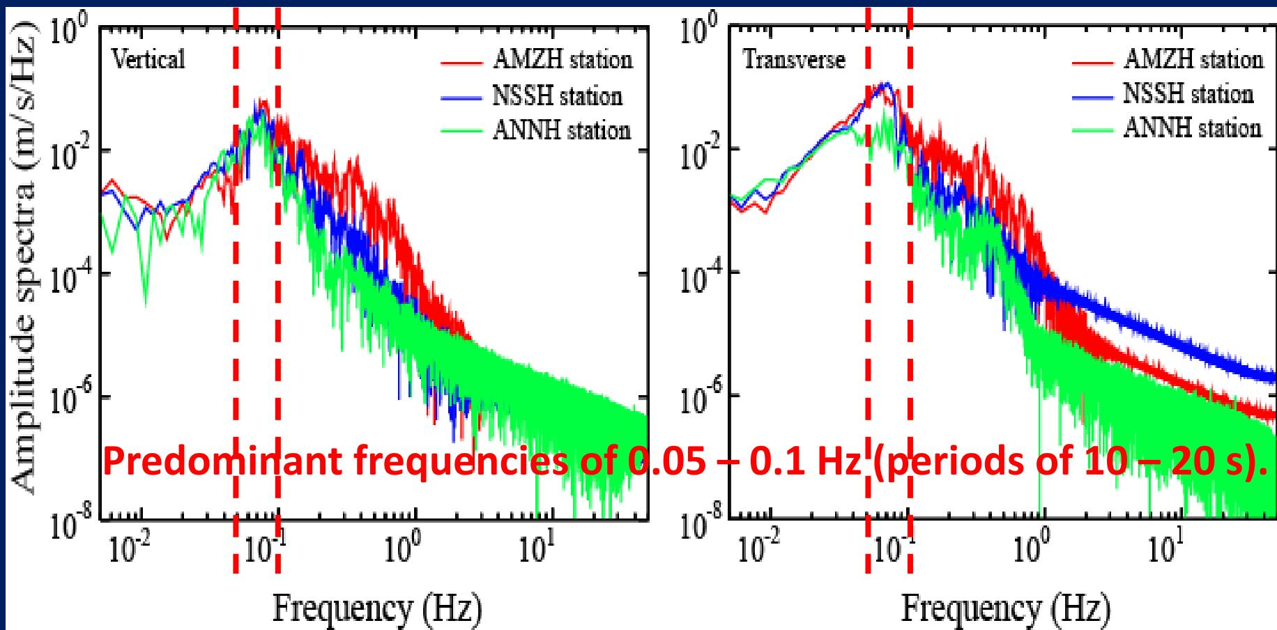
Velocity spectra for the **vertical** (left) and **transverse** (right) waveform components at the Hi-net stations AMZH (red), NSSH (blue) and ANNH (green) during a 500 s window, starting 10 s before the observed surface wave arrival.
