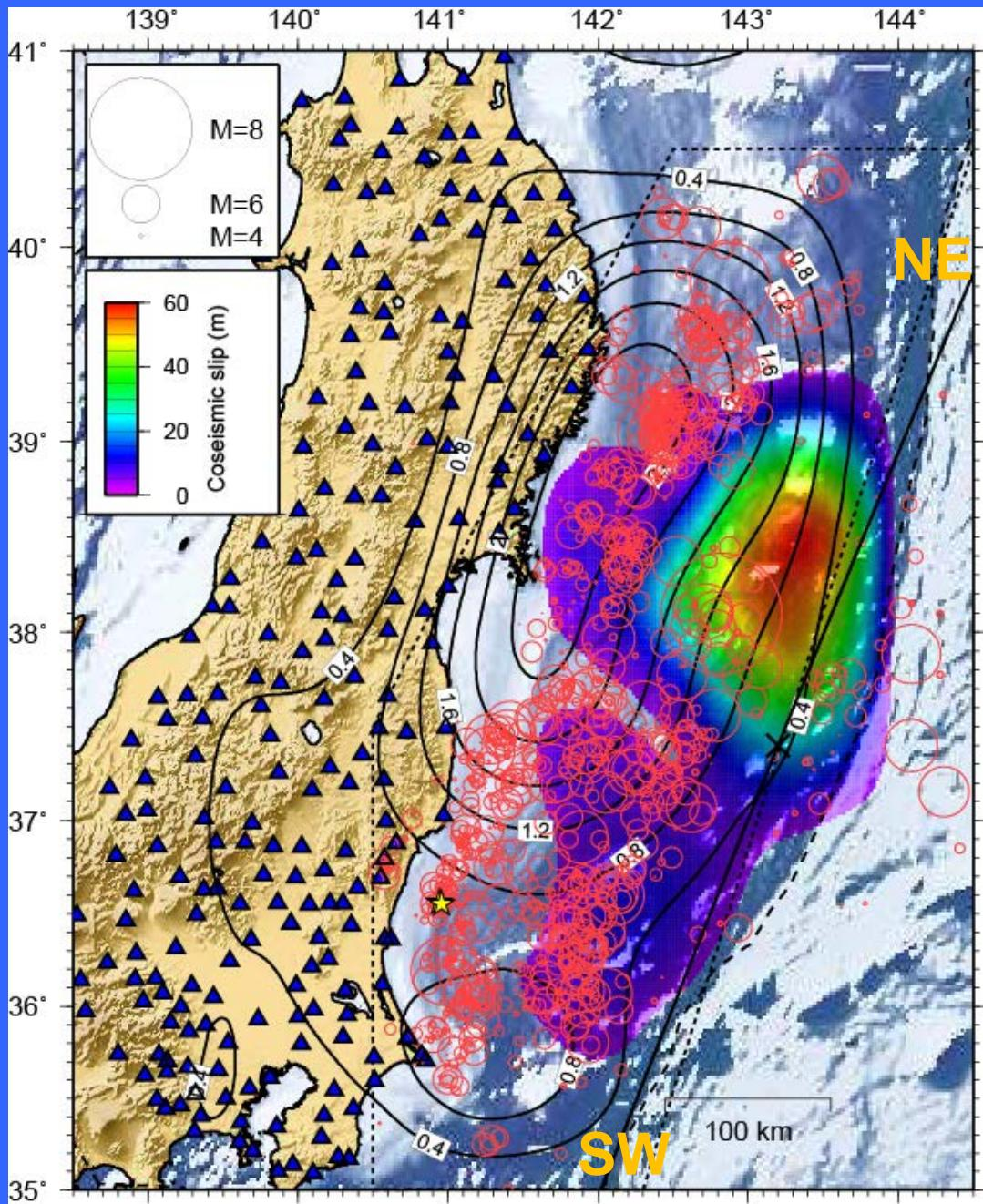
Decay and expansion of the early aftershock activity, following the 2011, Mw9.0 Tohoku earthquake
