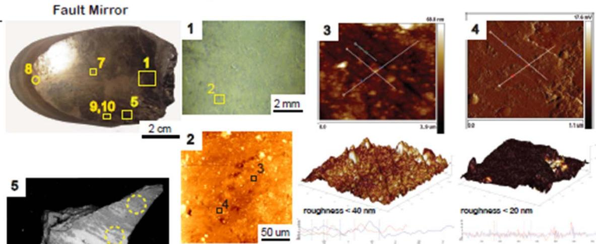
★ Smooth surface of FMs from the observation of (1) Optical and (2-4) AFM
