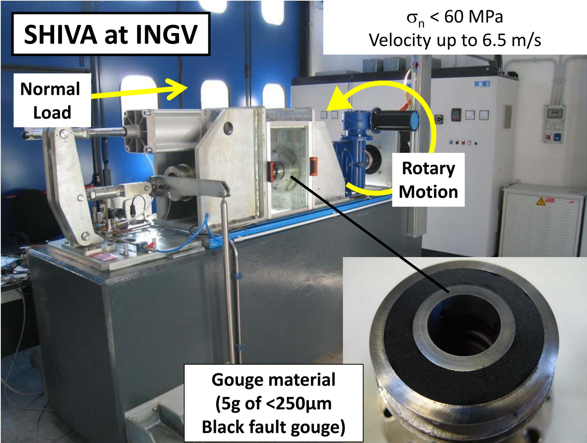
Tested up to **25 MPa normal stress** and  $3 \text{ m s}^{-1}$  slip velocity
