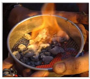
Combustion of gas hydrate recovered from UBGH1 (UBGH1 scientists, 2007)
