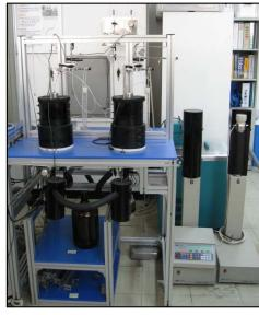
P-wave velocity measurement equipment
