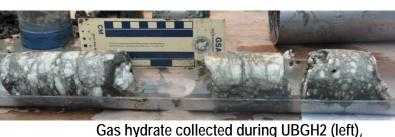
gas hydrate sample for bound water analysis (right)
