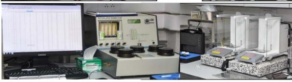
MAD pycnometer (left) & weighing balance (right)
