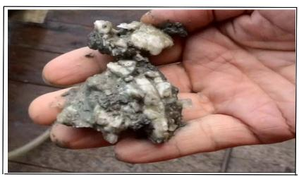
Gas hydrate recovered by using piston corer (KIGAM, 2007)
