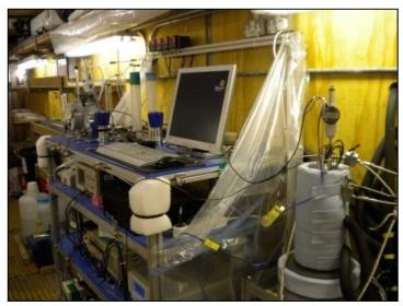
Gas hydrate production test using GHOBS (built by Dr. J.Y. Lee of KIGAM)
