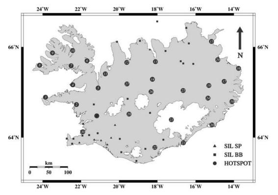
Figure 2. Map showing the locations of temporary (HOTSPOT) and permanent (SIL) seismic networks that were operational at the time of the Bárdarbunga earthquake (SP, short-period stations; BB, broad-band stations).
