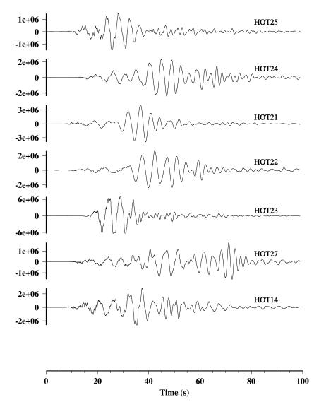
Figure 3. Vertical component velocity waveforms of the Bárdarbunga earthquake recorded at the closest (<150 km) HOTSPOT stations. The seismograms are arranged in order of increasing azimuth around the source (amplitudes in arbitrary units). Note the emergent onset and low-frequency content apparent at all stations around the source.
