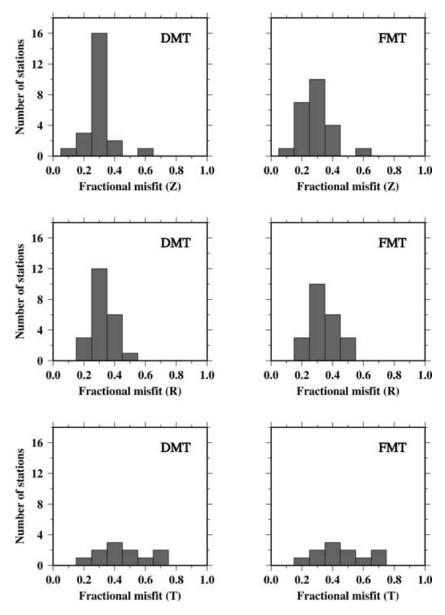
Figure 7. Histograms showing the distribution of the fractional misfits for each component (*Z*, vertical; R, radial; T, transverse) at all HOTSPOT stations for the inversion at 3.5 km depth (DMT, deviatoric moment tensor; FMT, full moment tensor) without distance-dependent weighting. The small number of transverse components is a result of many of them being excluded from the inversion because of contamination with long-period noise.
