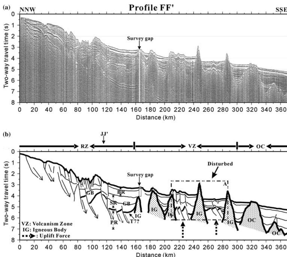
Figure 4. (a) Seismic profile FF' and (b) the interpretation of profile FF'. There are many intruded and extruded igneous bodies (IG) in this profile. Tilted, rotated normal faults are found near the basement. OC: oceanic crust. GB: graben. PR: pre-rift. SR: syn-rift. BR: post-rift.
