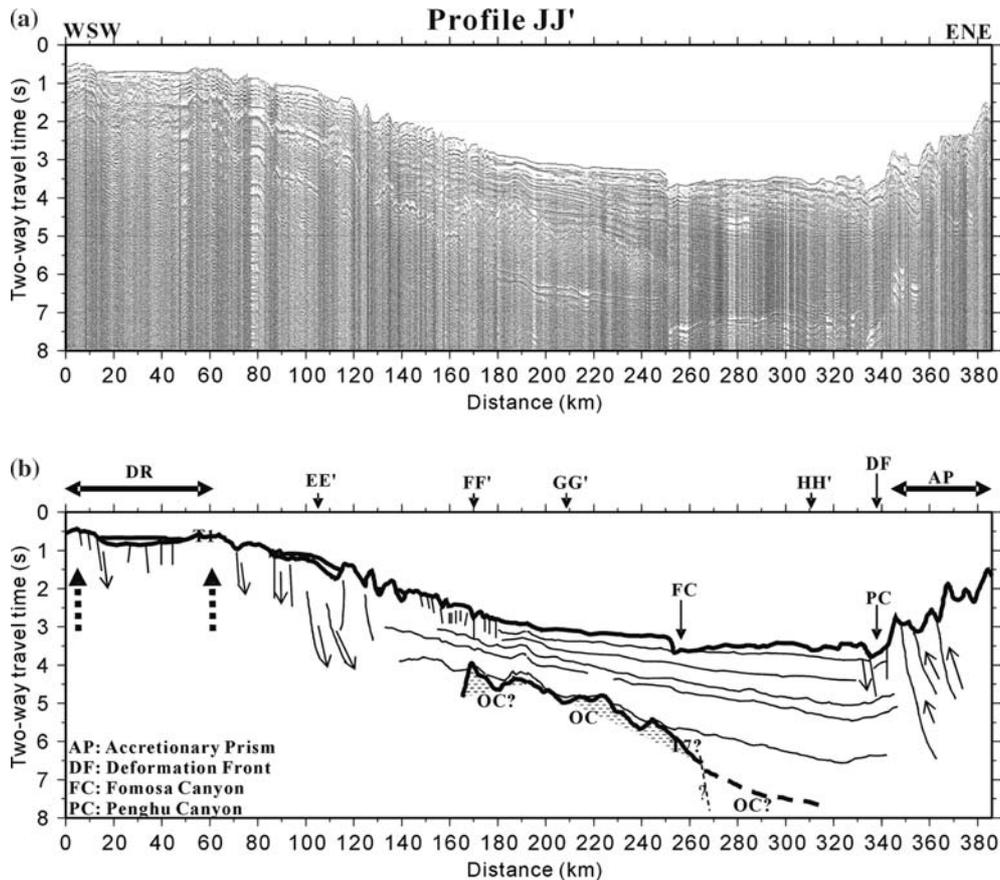
Figure 7. (a) Seismic Profile JJ' and (b) the interpretation of Profile JJ'. Uplift is seen near Dongsha Island. The basement progressively deepens from WSW to ENE. The basement is overlain by thicker sediment in the eastern part of the Formosa Canyon.
