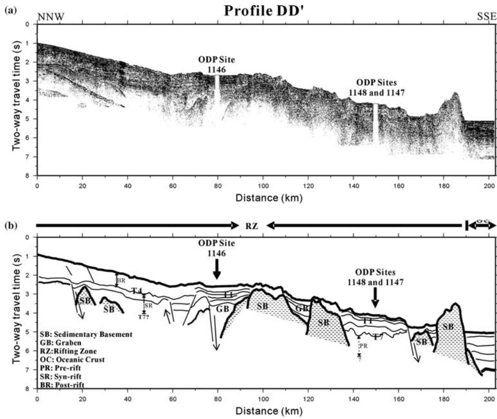
Figure 3. (a) Seismic Profile DD' and (b) the interpretation of Profile DD'. This profile is modified from Lüdmann et al. (2001). Several grabens filled with thick sediments are observed.
