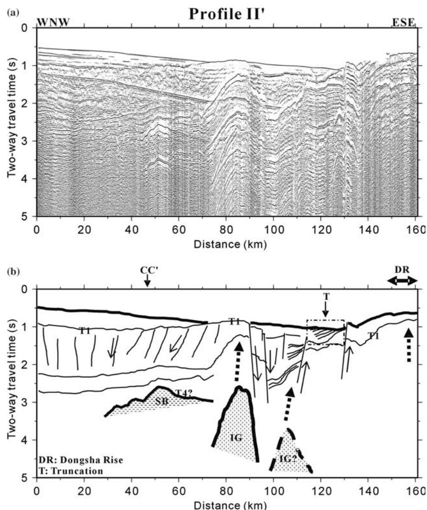
Figure 6. (a) Seismic Profile II' and (b) the interpretation of Profile II'. This profile displays many normal faults below the discontinuity T1. Intruded igneous rock is found at about 80 km distance and has caused topography uplift. Sediment truncation exists close to Dongsha Island (box T). DR: Dongsha Island.
