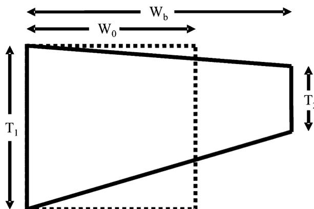
Figure 11. Diagram showing the original crustal block of length  $W_0$  and the stretched block of length  $W_b$ .  $T_1$ : the original continental crust thickness.  $T_2$ : the thickness of the thinned continental crust at the COB.
