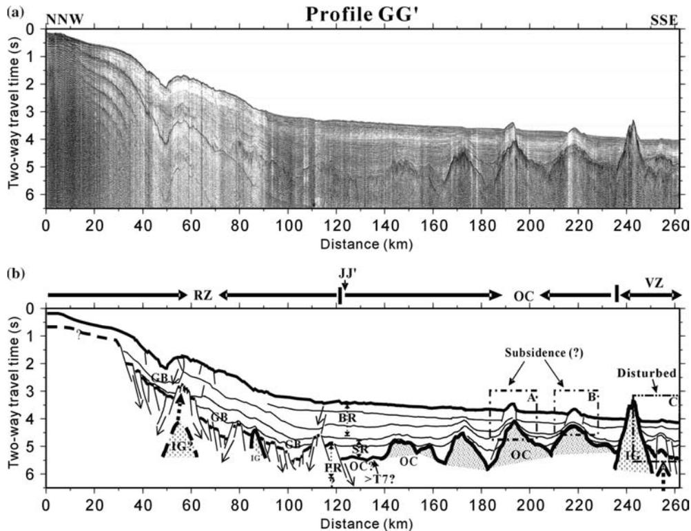
Figure 5. (a) Seismic Profile GG' and (b) the interpretation of profile GG'. There are many normal faults in the continental margin. Oceanic crust is found southward of the distance 130 km. IG: igneous body. OC: oceanic crust. GB: graben. PR: pre-rift. SR: syn-rift. BR: post-rift.
