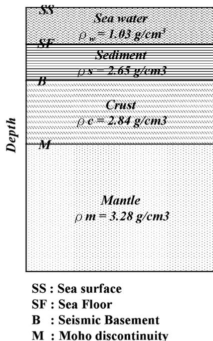
Figure 2. A simple four-layer crust model used for gravity modeling in this study.
