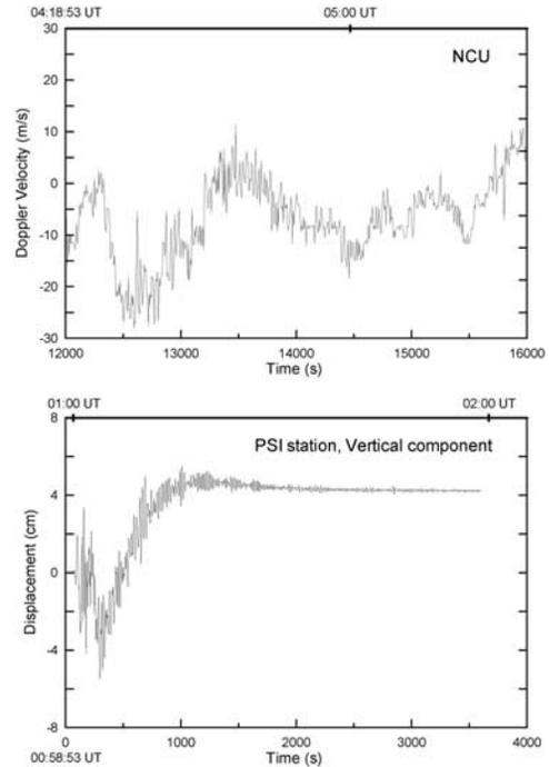
**Figure 3.** (top) Enlarged portion of the Doppler sounder record obtained at NCU, showing a big pulse of 30-minute duration. (bottom) Vertical ground displacement record obtained at the broadband seismic station PSI, showing a big transient followed by a permanent uplift of about 4 cm.
