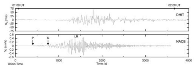
**Figure 4.** (top) Enlarged portion of the Doppler sounder record obtained at DHIT, showing oscillatory ionospheric disturbances. (bottom) Time histories of the vertical ground velocity obtained at NACB. The arrival times of P, S, and LR (Rayleigh) waves are marked on the trace.
