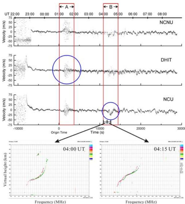
**Figure 2.** (top) Digital Doppler sounder records of the ionospheric disturbance obtained at stations NCNU, DHIT, and NCU. The circled portions of NCU and DHIT are enlarged in Figures 3 and 4, respectively. (bottom) Ionosonde records obtained at station HSS at 04:00 UT and 04:15 UT.
