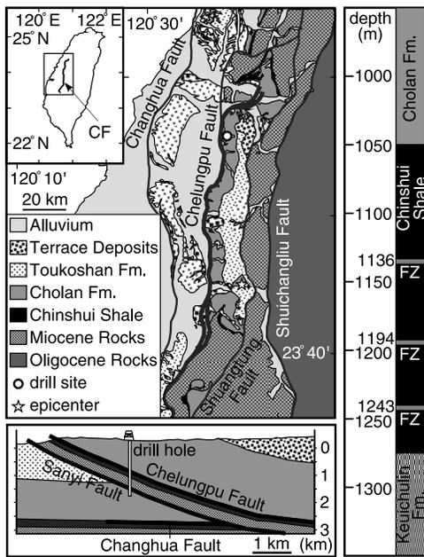
**Figure 1.** Geological map of central Taiwan, showing the site of the Taiwan Chelungpu-fault Drilling Project, an E-W cross section through the site location, and the lithological column of core samples recovered from Hole B [from Hirono et al., 2006]. CF, Chelungpu Fault; FZ, fault zone.
