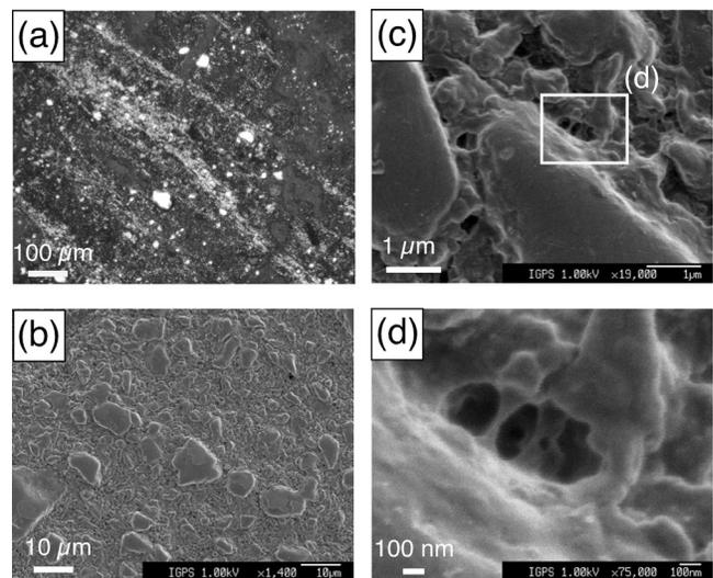
**Figure 4.** Microstructural observations of the BM disk in 1194mFZ. (a) Optical microscope image. (b) Scanning electron microscope image. (c) High magnification scanning electron microscope image. Hourglass structure can be seen on the edge of the large grain in the center of the image. (d) High magnification scanning electron microscope image. Hourglass and bubble structures can be seen in the center of the image.
