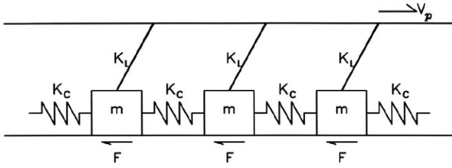
Fig. 1. An N-degree-of-freedom dynamical spring-slider system.
