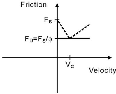
Fig. 2. Schemes for the constant dynamical frictional force (solid line) and the velocity-dependent weakening-hardening frictional force (dashed lines).  $F_s$  is the static frictional force;  $\phi$  is the ratio of static to dynamic frictional forces;  $V_c$  is the critical velocity having the lowest frictional force.
