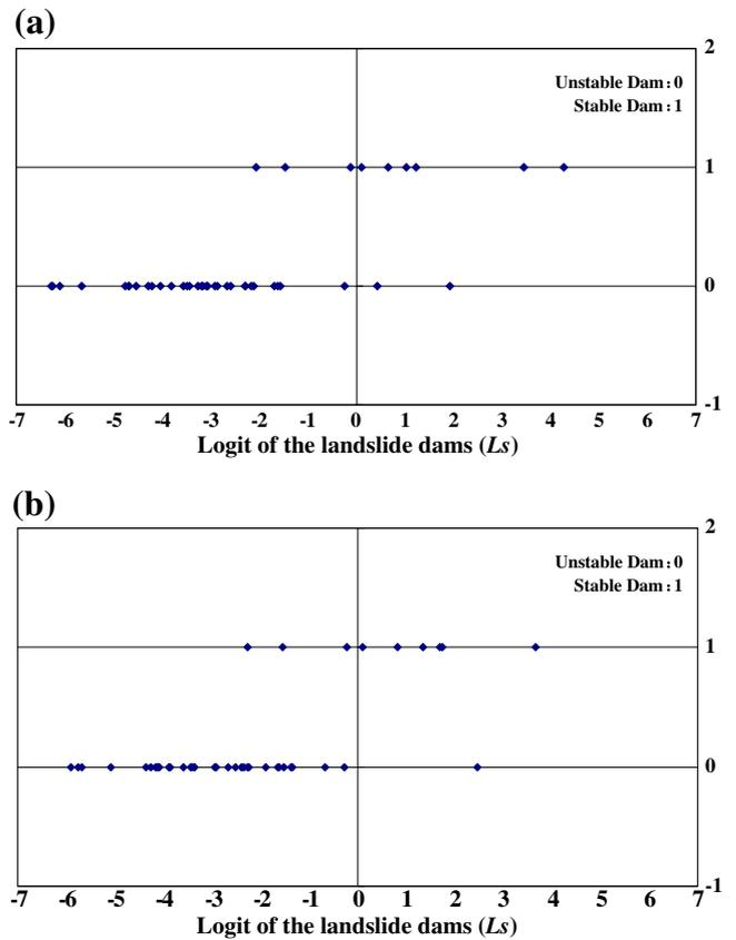
Fig. 1. Logit (*L<sub>s</sub>*) distribution (*L<sub>s</sub>* > 0 stable, *L<sub>s</sub>* < 0 unstable) of (a) the Model PHWL\_Log, and (b) the Model AHWL\_Log for the stability of 43 landslide dams.
