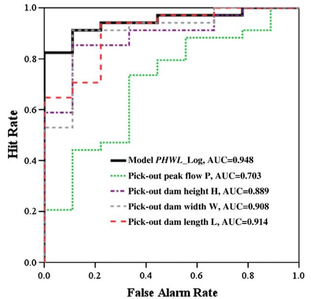
Fig. 3. ROC curves of Model PHWL\_Log and 4 sub-models.
