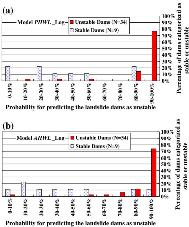
Fig. 5. Histogram showing the distribution of failure probability ( $P_f$ ) of the 43 landslide dams. (a) Model PHWL\_Log; (b) Model AHWL\_Log.
