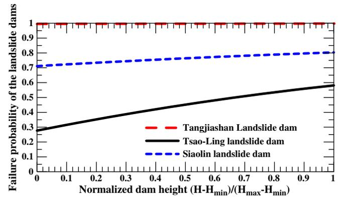
Fig. 8. The sensitivity analysis for the dam height on the failure probability of Tsao-Ling and Tangjiashan landslide dam using Model *AHVL\_Log*.
