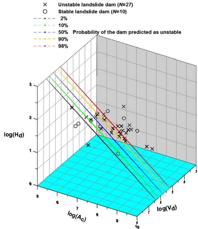
Fig. 6. Contour planes for 2%, 10%, 50%, 90%, and 98% of failure probability of a landslide dam predicted by the Model AHV\_Log. The stable and unstable landslide dams in Tabata's inventory (37 target dataset) and the failure probability of Tangjiashan and Tsao-Ling landslide dam are also shown.
