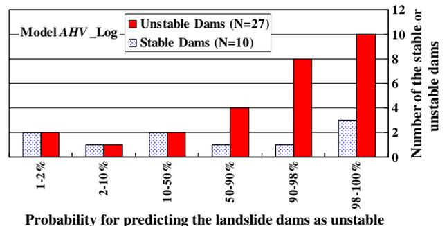
Fig. 7. A comparison of relative frequencies of stable and unstable landslide dams of the target data set (37 Japanese cases) and dam failure probabilities ( $P_f$ ) calculated from the Model AHV\_Log developed from the training data set (84 worldwide cases).
