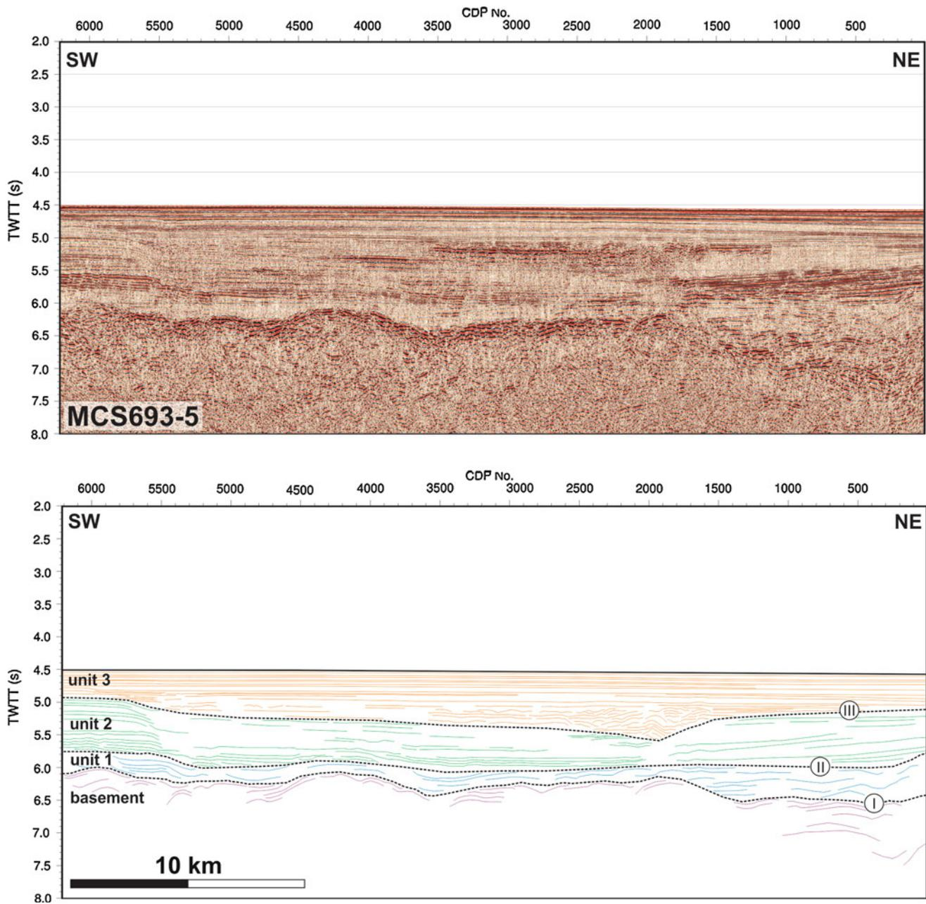
**Fig. 4** (Top panel) Multi-channel seismic profile MCS693-5. (Bottom panel) Interpreted section. Very wide submarine channels are identified in the section. The unconformities show minimal relief
