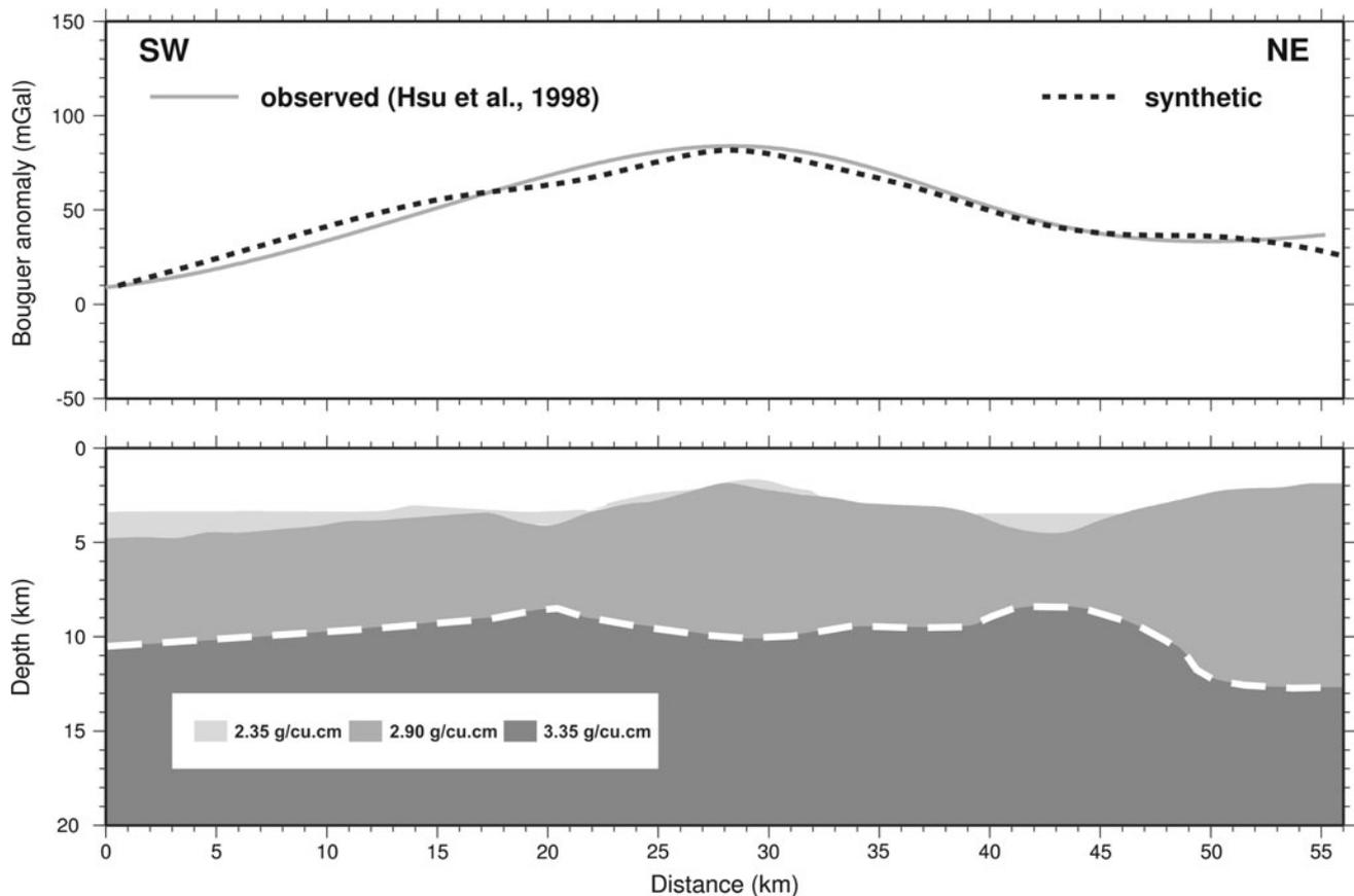
**Fig. 6** Gravity model coincident with the seismic profile MGL0908-25. The model shows the shallow roots for the region and the prevailing isostatically uncompensated state of the active zone. *Thick dashed white line* delineates the modeled Moho boundary
