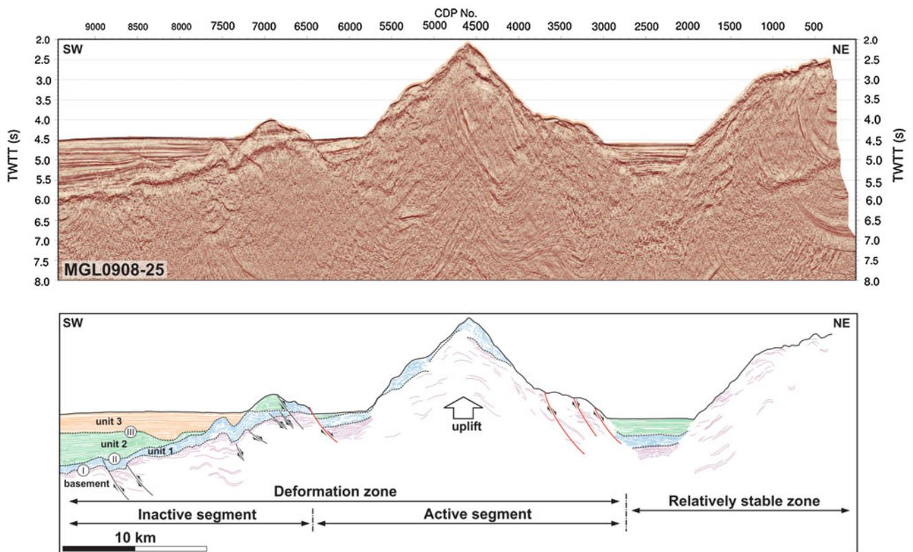
**Fig. 5** (Top panel) Multi-channel seismic profile MGL0908-25. (Bottom panel) Interpreted section. The study area is divided into deformation zone and a relatively stable zone. The zone of deformation
