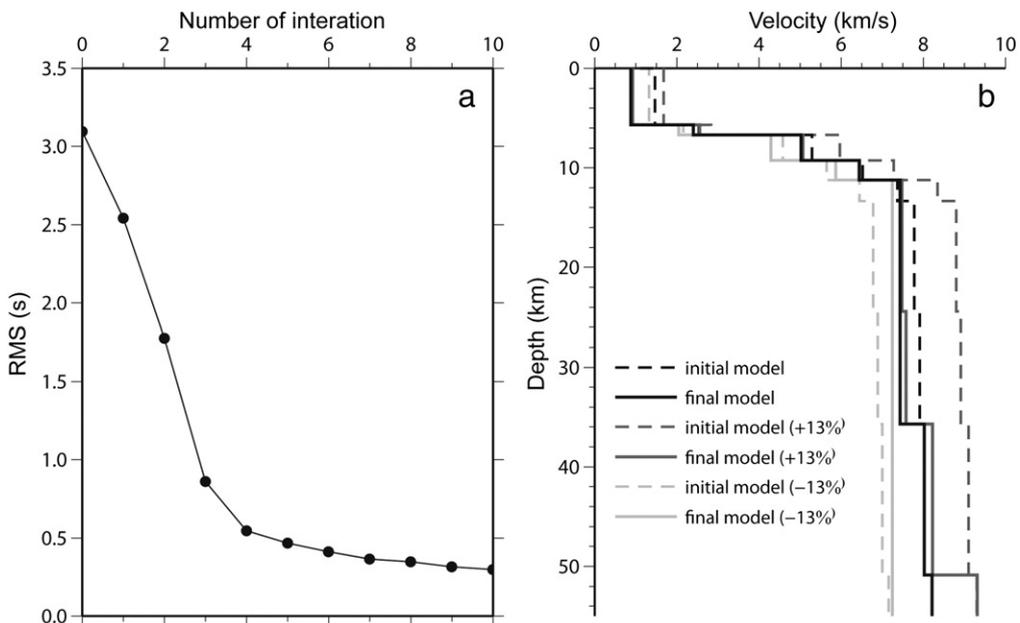
**Fig. 3.** (a) RMS distribution as a function of the number of iterations during the 1-D velocity inversion using the VELEST program. (b) Initial input velocity model (dashed lines) and their corresponding inverted model (solid lines). The inversion was performed by varying the initial velocity value by  $\pm 13\%$ .
