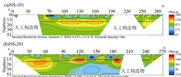
**Figure 7. The resistivity image collected along the north-south direction in the Choushuichi upper fan area, including. (a) NS-101; and (b) NS-201**
