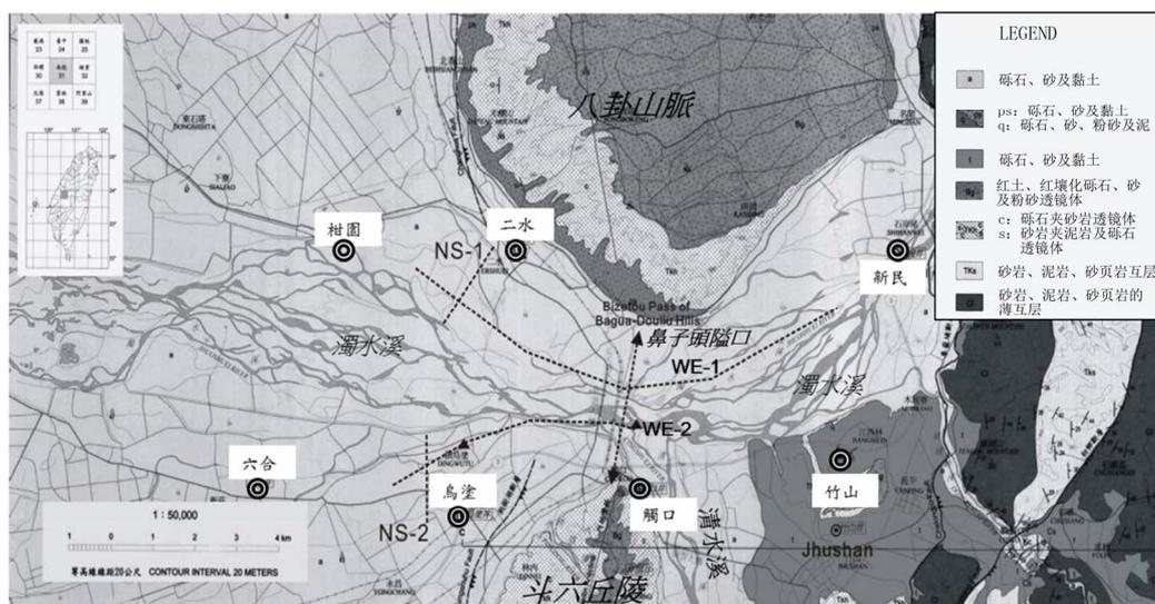
Figure 1. Locations of the observation wells and resistivity survey designs in the upper Choushui Alluvial Fan
