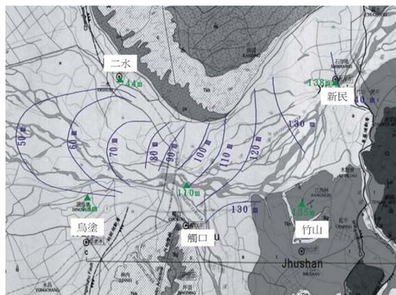
Figure 8. The groundwater surface in the unconfined aquifer constructed from the data of resistivity measurements and the water level in the observation wells(green triangles).
