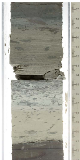
Figure F14. Two calcareous turbidites stacked on top of one another, Hole U1433B (48R-1A, 56–73 cm). The lower turbidite is finer grained claystone to siltstone with a Chondrites -burrowed top. The upper turbidite is silty and laminated with larger Planolites burrows, grading upward into claystone.
