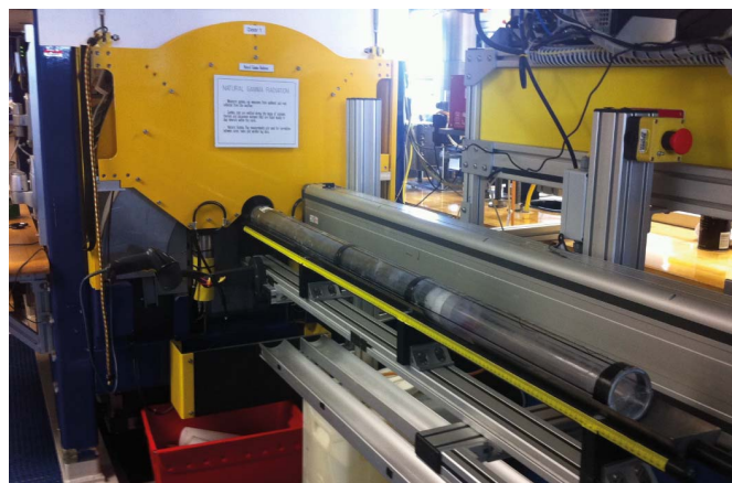
Figure F31. NGRL for whole-round cores, which conducts 8 measurements at a time in 2 positions, resulting in 16 measurements per core.
