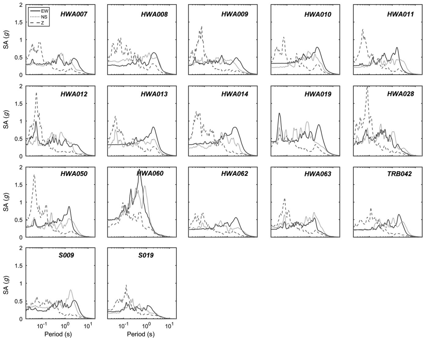
▲ **Figure 8.** Three components of spectral accelerations at the 17 stations that recorded pulse-like velocities. Solid, dotted, and dashed curves represent the east–west, north–south, and vertical components, respectively.
