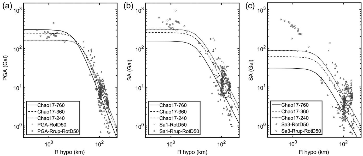
▲ **Figure 3.** Comparison of observed strong motions and those estimated from the Chao *et al.* (2017; referred to as Chao17) ground-motion prediction equation (GMPE), assuming  $V_{S30} = 240, 360,$  and  $760$  m/s: (a) PGA, (b) spectral acceleration at 1 s (SA1), and (c) spectral acceleration at 3 s (SA3). Rrup was used to find the circles and hypocentral distance for the triangles.
