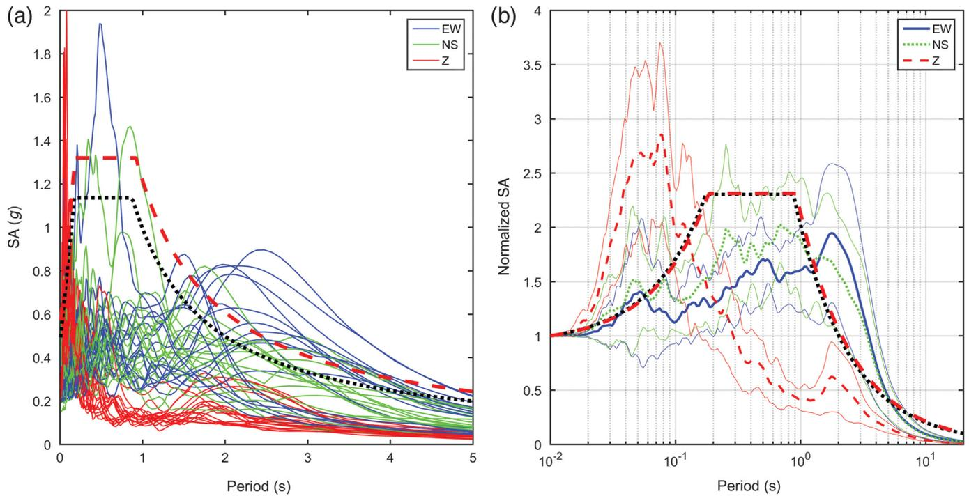
▲ **Figure 9.** (a) Superposition of the spectral accelerations at the 17 stations that recorded pulse-like velocities and the design spectra (black and red dotted lines). (b) Average three-component spectral accelerations at 16 stations.
