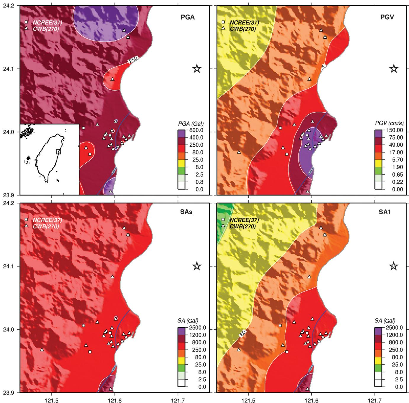
▲ **Figure 2.** Spatial distribution of intensity measures (peak ground acceleration [PGA], peak ground velocity [PGV], spectral accelerations [SAs], and SA1) in the Hualien region during the mainshock. The inset in lower left of the PGA map indicates Taiwan island and the frame (black rectangle) of this figure.
