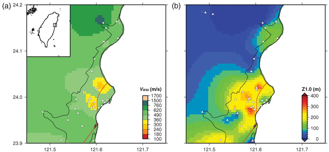
▲ **Figure 4.** Distributions of (a)  $V_{S30}$  and (b)  $Z_{1.0}$  in the Hualien region. The inset in upper left of the  $V_{S30}$  map indicates Taiwan island and the frame (black rectangle) of this figure.
